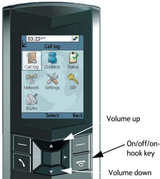
If the handset does not start up, the reason may be that there is no PoE in the LAN interface. If you are connecting to a BGAN terminal, check that the PoE indicator on the terminal lights green for the connected port. For further information, refer to the installation manual for the BGAN terminal.
