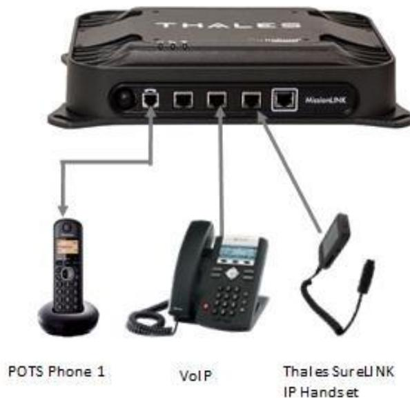
*Figure 2-3 Thales SureLINK Handset Connected to TU /BDU*
