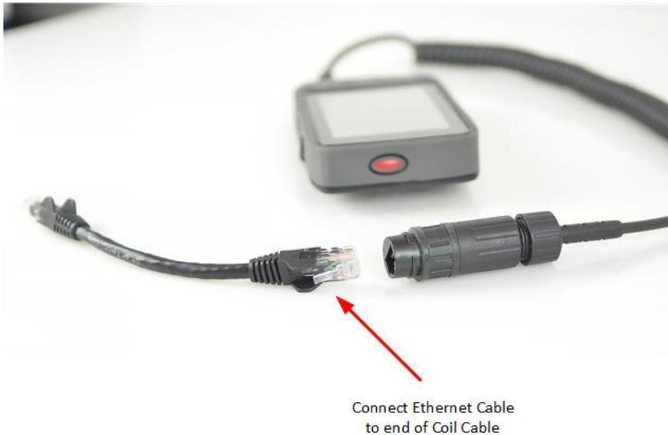
*Figure 2-2 Ethernet Cable Connection to Handset*
