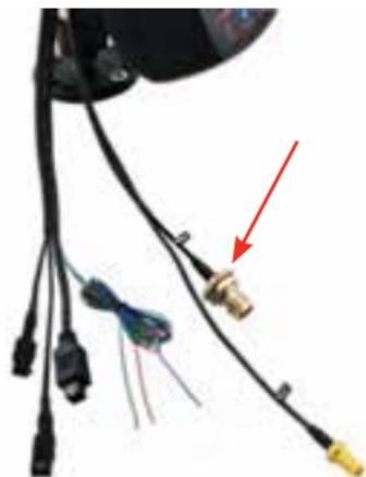
The antenna connections exit from the rear of the SatDOCK-G 9555 cradle, via the antenna loom as shown in the picture.
