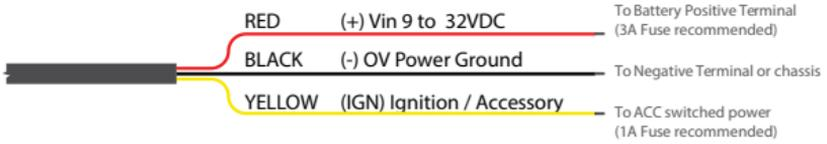
5. Connect the **YELLOW** wire to the vehicle accessory power. If the accessory power is unavailable, this may be connected to a vehicle ignition voltage. It is recommended to add a 1A fuse between them. The accessory wire enables the SatDOCK-G 9555 to turn on and off as the vehicle key is enabled or disabled. If this function is not required, the **YELLOW** wire **MUST** be connected to the **RED** wire.
