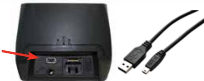
To connect a PC/laptop to the SatDOCK-G 9555 bottom mini-USB port, you will require a mini-USB-B to USB-A data cable. This cable is included in your original 9555 package.
