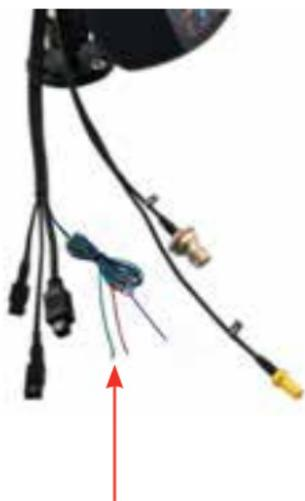
SatDOCK-G 9555 provides an additional cable pair from its rear cable loom, known as the standard Beam alarm loop. This provides a Normally CLOSED wire loop, which can be used to connect to any passive type of button, or relay, or reed switch in which the action breaks the loop (OPEN) to activate the alarm state.
