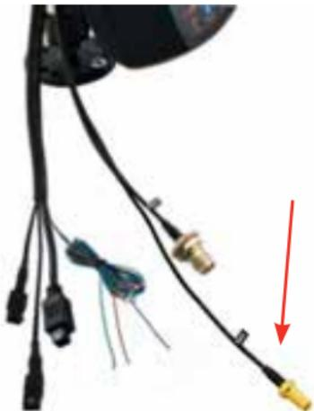
The GPS connection is optional if the tracking function is required. If connected, and tracking is enabled, position or location information will be shown on your tracking messages and alert messages.
