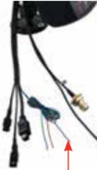
The SatDOCK-G provides a **BLUE** wire output on the rear cable loom for controlling an external ringer such as a vehicle horn.
