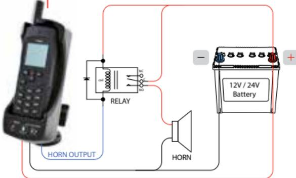
By default, it only works when the key ignition is OFF and the SatDOCK-G is still ON (by default, the SatDOCK-G will stay on for 20 minutes after the key ignition is turned OFF). This is to avoid the horn buzzing on an incoming call while the vehicle is being driven.
