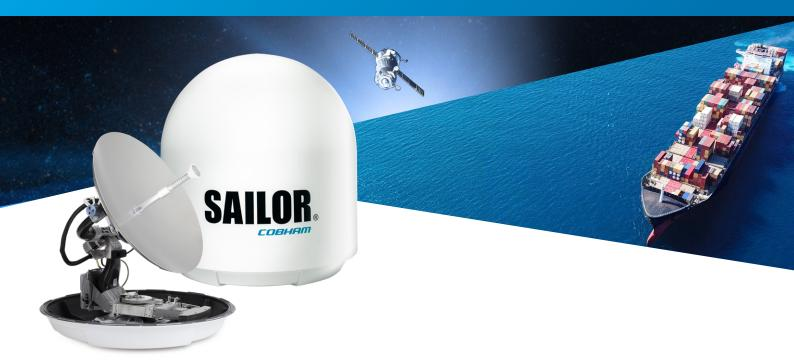
Your compact and lightweight future-proof Ka-band system for Inmarsat Global Xpress® — available with either 4.5W or 9W wideband, dual-pol transceiver.
