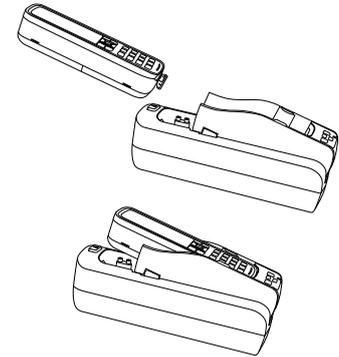
4. To remove the handset from the cradle, press the EJECT button at the top of the docking station. The dock will swing out and the handset can be removed.
