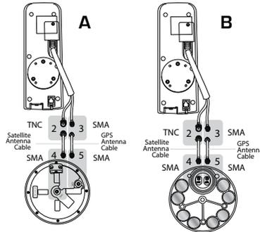
**A** - Connection with Fixed/Directional Antenna (Passive)
