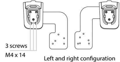
3. Mount the spacer plate and the mounting bracket to the rear of the IsatDock LITE, by using the longer screws provided with the kit. The original RAM® arm-bracket plate is also re-installed behind these plates. Install in the following order:
