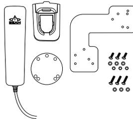
2. Mount the handset cup to the mounting plate, it can be installed to the left or right side of the dock by simply rotating the bracket. Secure the cup with the washer and nut bolt behind the bracket.
