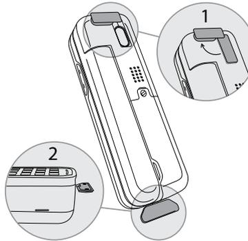
3. To dock the handset, align the IsatPhone Pro with the phone tray and slide the handset down until it seats flush to the bottom of the tray. Swing the phone down into the
