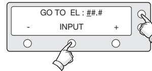
5. Input position value for elevation (EL) axis.
