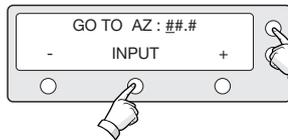
4. Input position value for azimuth (AZ) axis.
