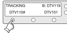
2. The antenna is tracking Satellite B.
