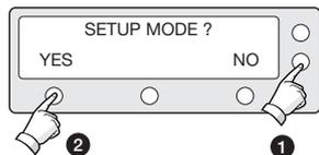
1. Enter "SETUP MODE" Press the Right Lower Vertical button indicated as "1".
