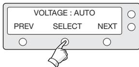
17. Select the **Voltage Supply Method\*** to LNB.
