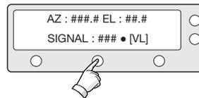
5. Antenna position detail and signal strength are displayed.
