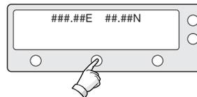
6. Press center soft key to display current GPS information. Press center soft key to return to main tracking mode.
