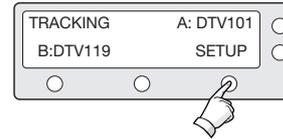
1. While the antenna is tracking press SETUP
