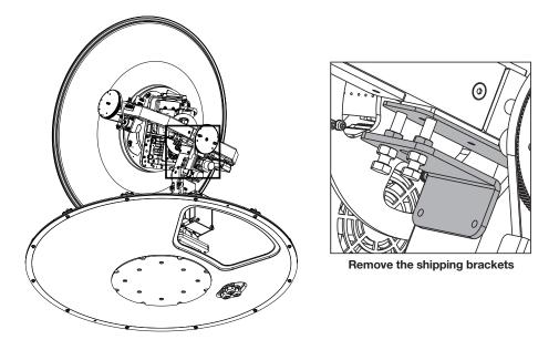
C. Re-assemble the top radome and tighten the radome retention bolt (M6) to a torque setting of 3.5 N·m. To ensure security, apply Loctite #242 or equivalent.
