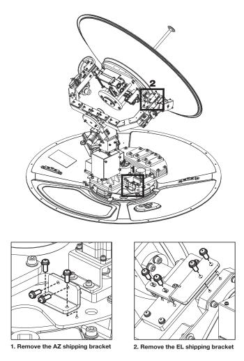
B. Remove the shipping brackets securing the CL axis.
