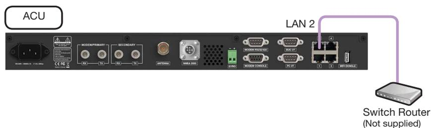
Figure: ACU to Switch Router Cable Connection
