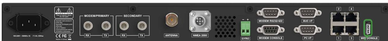
Figure: Rear Panel Wi-Fi Dongle Connection
