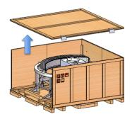
Remove the fixing screws from the panels, and then detach the panels in order (① left panel → ② back panel → ③ right pane).
