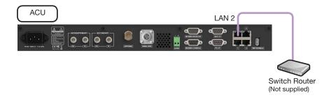
Figure: ACU to Switch Router Cable Connection
