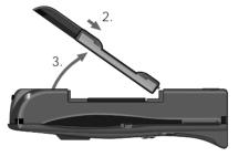
**4. Insert the battery**, bottom-end first, into the compartment, and then press the battery downward until it clicks into place.
