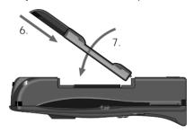
**8. Replace** the battery cover. See "Attach the Battery Safety Cover" on page 29.
