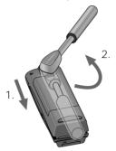
**2. Rotate the antenna** to either the left or right detente (the antenna will stop here).
