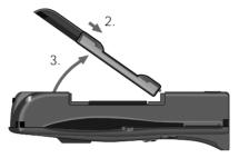
**4. Press and hold the release latch** at the top of the battery.
