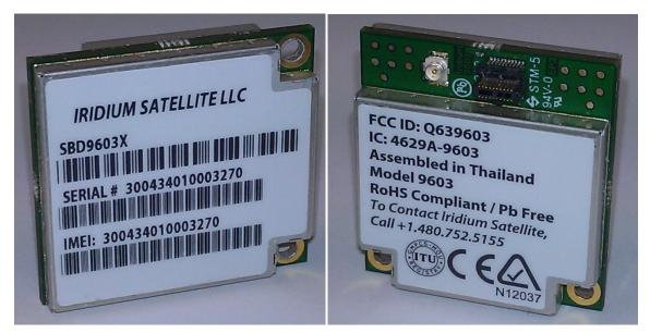
Figure 1. Iridium 9603 SBD Transceiver Front and Back Views (please note the 9603 may also reference FCC ID Q639603N and IC 4629A-9603N)
