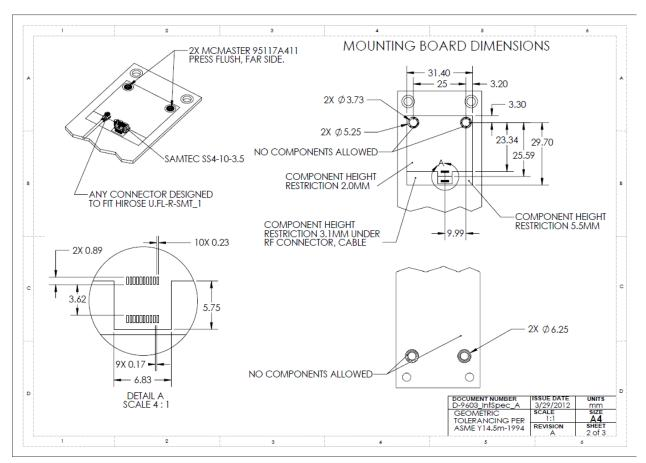
Figure 3. Motherboard mounting for the 9603 Transceiver
