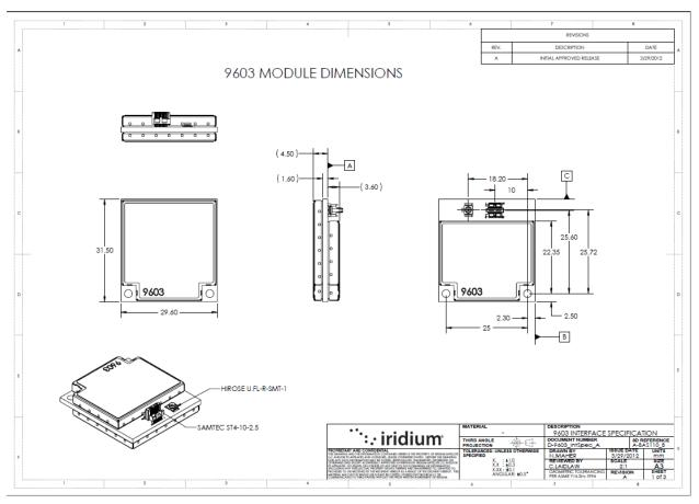
Figure 2. Dimensions of the 9603 Transceiver
