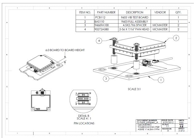
Figure 5. Motherboard mounting suggestions for the 9603 Transceiver
