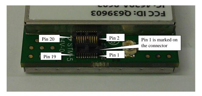
Figure 6. User Connector Pin Number Designation
