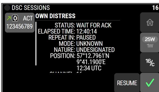
2. The radio watches for a DSC acknowledgment transmission on channel 70.
