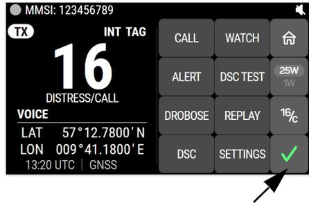
Tap the BAM icon to enter the alert list. The alert list is a list of all active alerts on the VHF. Each alert entry shows the alert state, using the appropriate icon, the alert title and alert buttons to interact with the alert.
