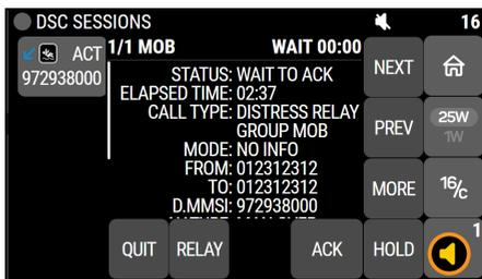
The MOB distress relay calls (closed loop) can be relayed or individually acknowledged when the person is located or secured.
