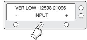
8. Input the tracking frequency (MHz) and symbol rate (KHz) for vertical low band.
