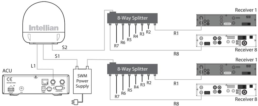
Figure 01 : Basic Configuration with 16 Receivers
