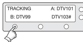
1. Press LEFT soft key for tracking Satellite B.
