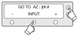
4. Input position value for azimuth (AZ) axis.
