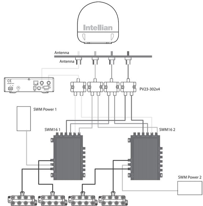
Figure 16 : 32 Receivers Connection
