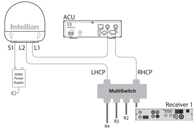
Figure 15 : 16 Receivers Connection
