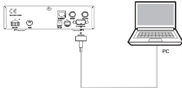
Figure 26 : Serial Connection
