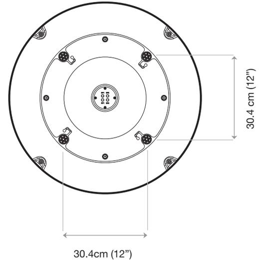
**Figure 09 : Mounting Hole Position of s6HD**
