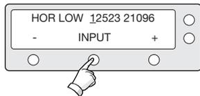
10. Input the tracking frequency (MHz) and symbol rate (KHz) for horizontal low band.
