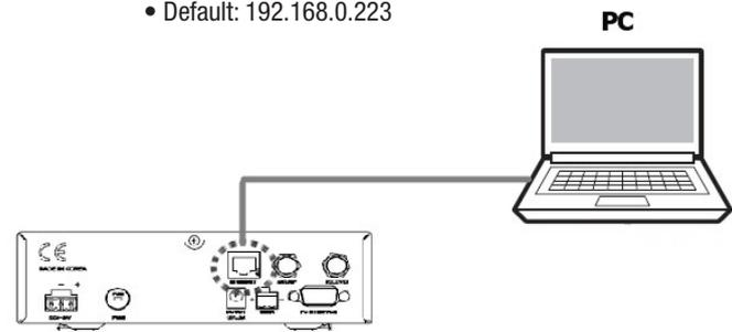
Figure 28 : ACU to PC TCP/IP Connection
