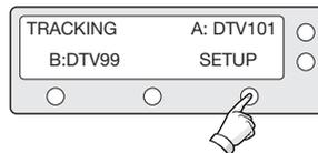
1. While the antenna is tracking press SETUP
