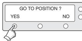
6. Press YES to move the antenna to input position.
