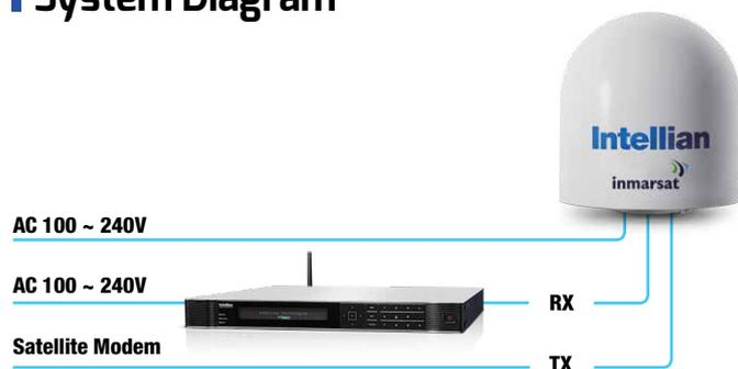
**Intellian v100GX** is a 1 meter Ku-band to Ka-band GX convertible maritime stabilized antenna, and ready-to-use system for the super-fast, Global Xpress™ (GX) Ka-band broadband service from Inmarsat.
