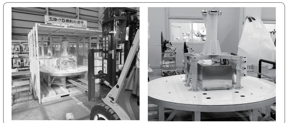
**Move Base Frame using Fork Lift**
