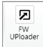
**FW Uploader:** launches firmware upload wizard to upgrade Antenna and ACU firmware from a PC. Connect the PC to the ACU via a USB cable and follow instructions on the Wizard until the firmware upgrade is complete.
