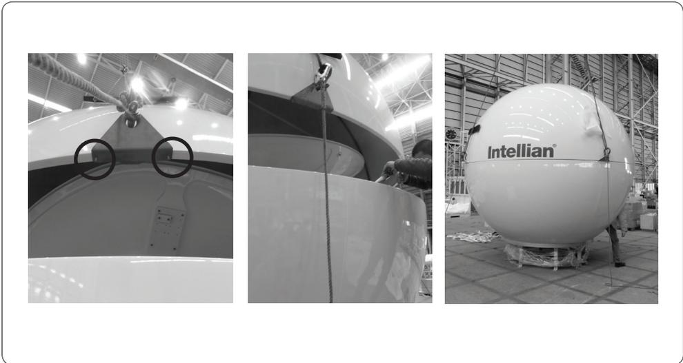
**Assemble the Upper Radome and the Lower Radome (II)**
