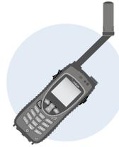
The antenna is fully extended and rotated towards the sky (signal strength will be indicated on the top left hand corner of the display). Ensure that the antenna is articulated left or right so it is oriented directly up when held to your ear during use.
