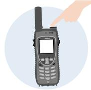
Power-on by pressing black button on the top of the phone for 5 seconds until the screen illuminates.
