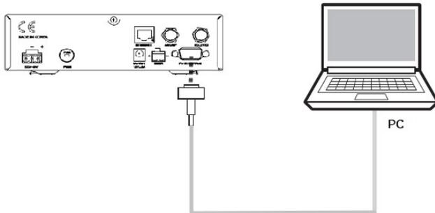
Figure 22 : Serial Connection
