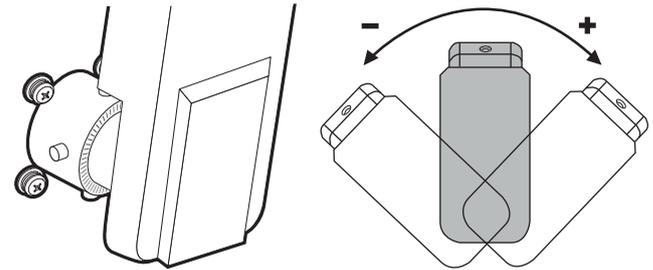
Figure 21 : Manual Angle Adjustment LNB Skew
