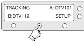
4. The antenna is again tracking Satellite A. Press center soft key to display position detail.
