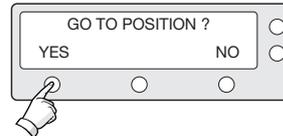
6. Press YES to move the antenna to input position.
