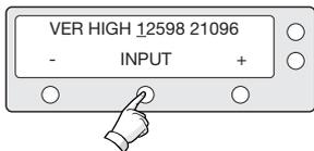
12. Input the tracking frequency (MHz) and symbol rate (KHz) for vertical high band.
