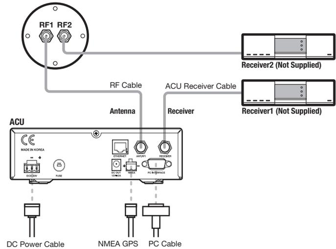
Figure 16 : Dual-Receivers Configuration
