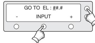
5. Input position value for elevation (EL) axis.
