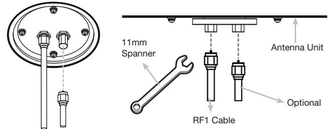
Figure 11 : Connectors on Bottom of Antenna
