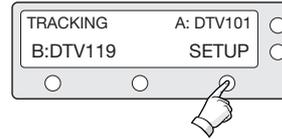
1. With the antenna is tracking, press SETUP.
