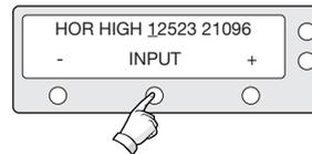
14. Input the tracking frequency (MHz) and symbol rate (KHz) for horizontal high band.
