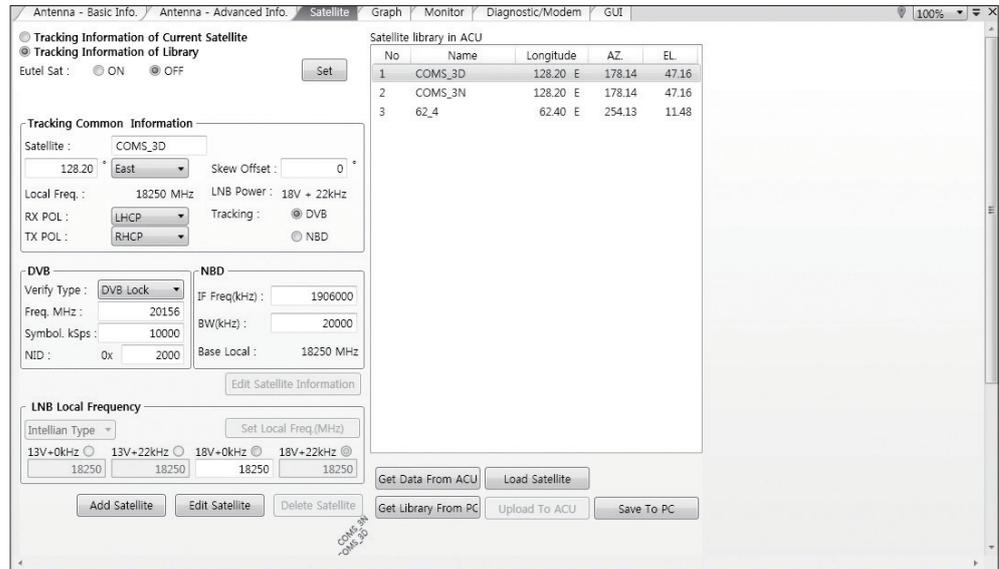
This view provides information on the Satellite's Information, Tracking Common Information, DVB and NBD Tracking Transponder, LNB Local Frequency, and Satellite Library. This view shows a graphic UI of the current satellite that the antenna is pointing at and the satellites that are located at a 180° arc on the horizon with reference to the current position.
