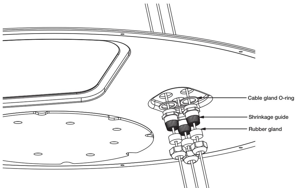
Cable connections on power switch box
