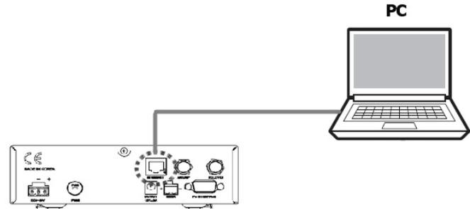
Figure 23 : ACU to PC TCP/IP Connection
