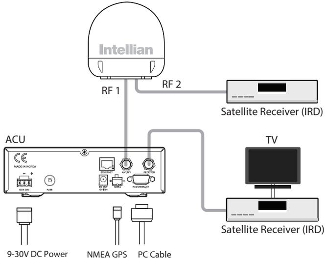
**Figure 1: Basic System Configuration**
