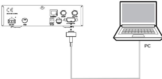
Figure 21 : Serial Connection
