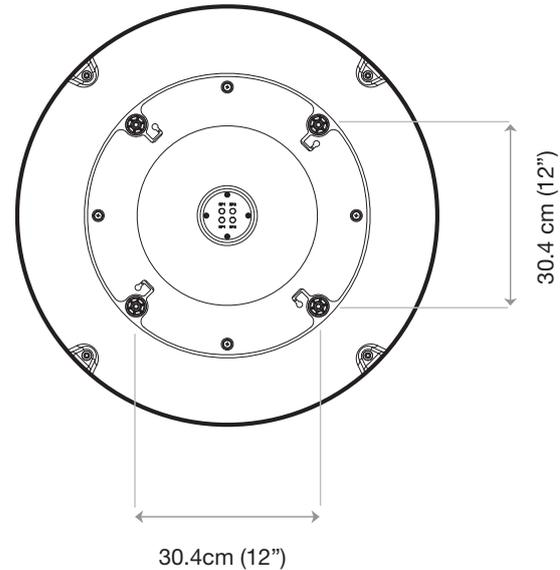
**Figure 9: Mounting Hole Position of i6W**
