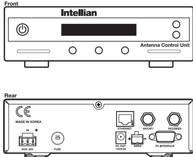
Figure 3: Antenna Control Unit (ACU)
