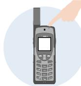
Power-on by pressing black button on the top of the phone for 5 seconds until the screen illuminates.
