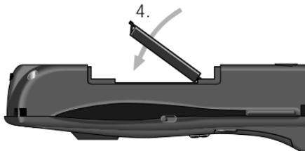
5. **Insert the bottom end** of the compartment cover into the slots at the end of the compartment.
