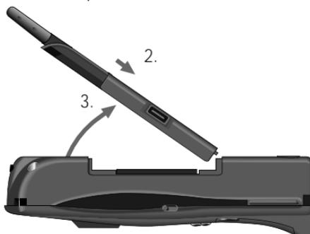
4. **Insert the bottom end** of the battery compartment cover into the slots at the end of the compartment.
