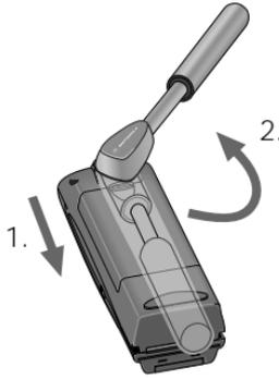
2. **Rotate the antenna** to either the left or right detente (the antenna will stop here).
